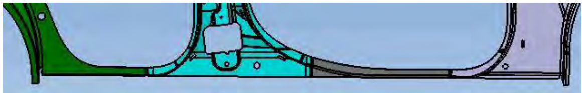
Figure 13.20: B-pillar lower portion (showing the feature for seat belt retention)
