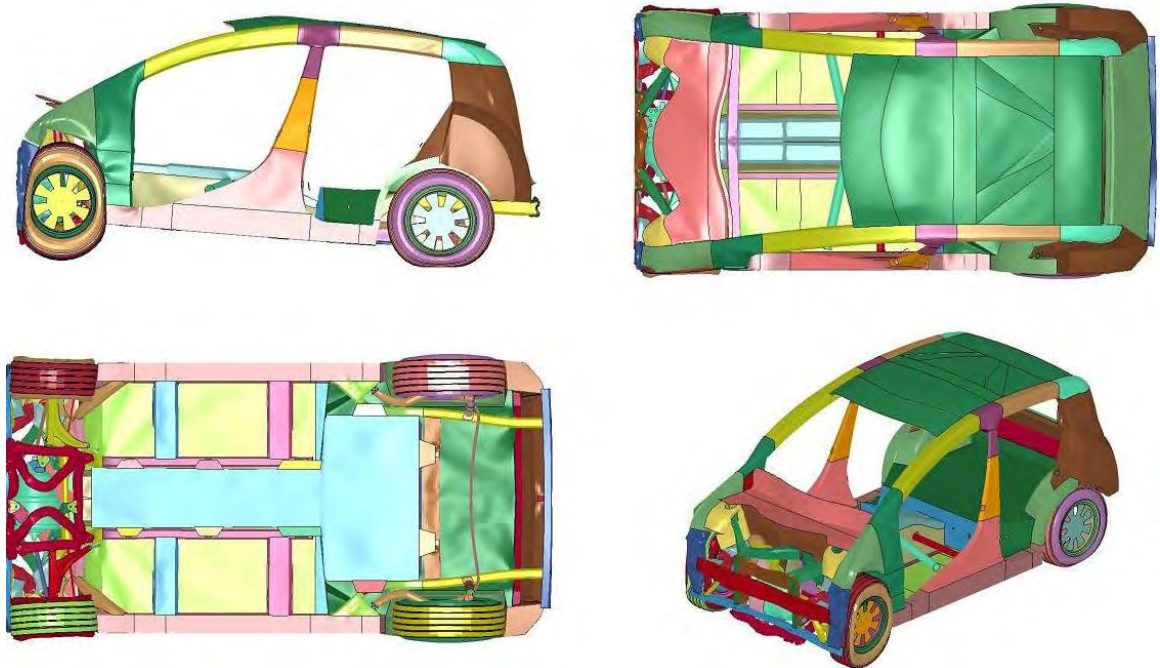
Figure 8.28: NCAP deformed shape : design 60
