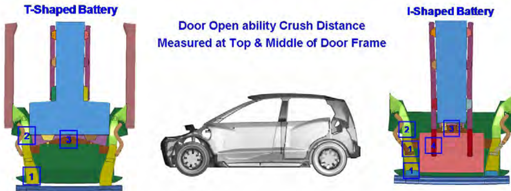
Figure 8.45: T-shape versus I-shape optimization result comparison
