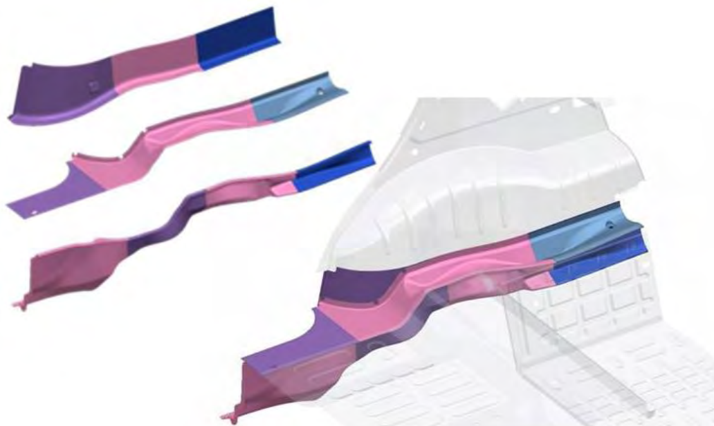
Figure 14.6: FSV rear rail - optimized sections
