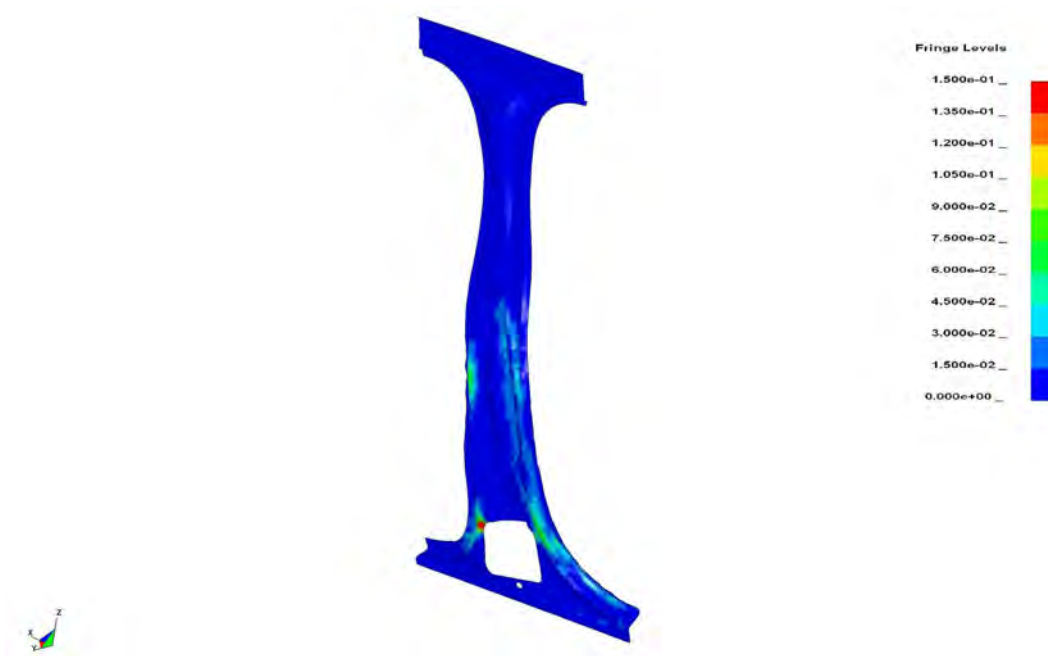
Figure 14.41: IIHS side impact - B-pillar inner (% plastic strain contour)
