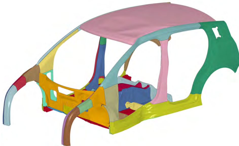
Figure 14.71: FMVSS 214 pole impact - FSV main load path components deformation at 100 ms post-pole test position
