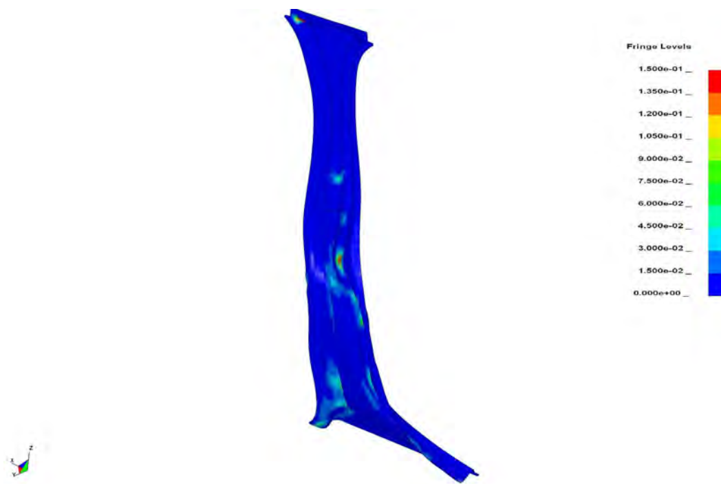
Figure 14.42: IIHS side impact - B-pillar reinforcement (% plastic strain contour)
