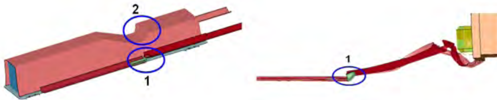
Figure 19.14: Battery pack before and after rear crash of original design
