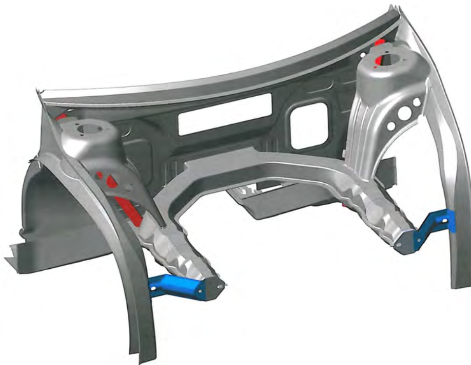
Figure 13.62: 50.1 3000 Front structure assembly
