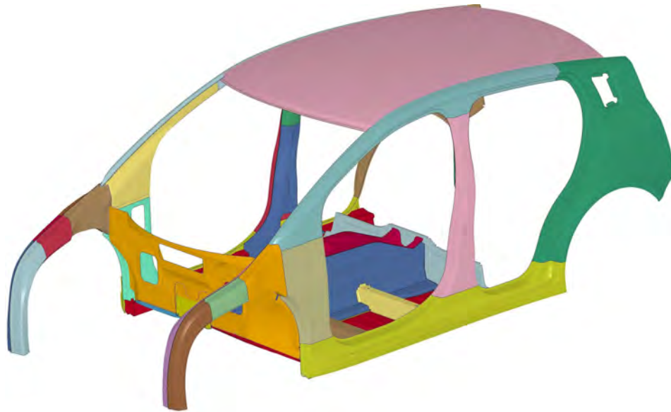
Figure 14.70: FMVSS 214 pole impact - FSV main load path components at pre-pole test position
