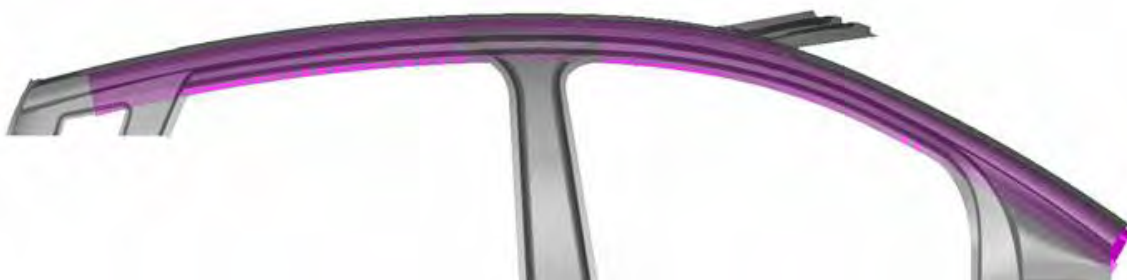
Figure 13.7: FSV Phase-2 T4 roof rail stamped solution
