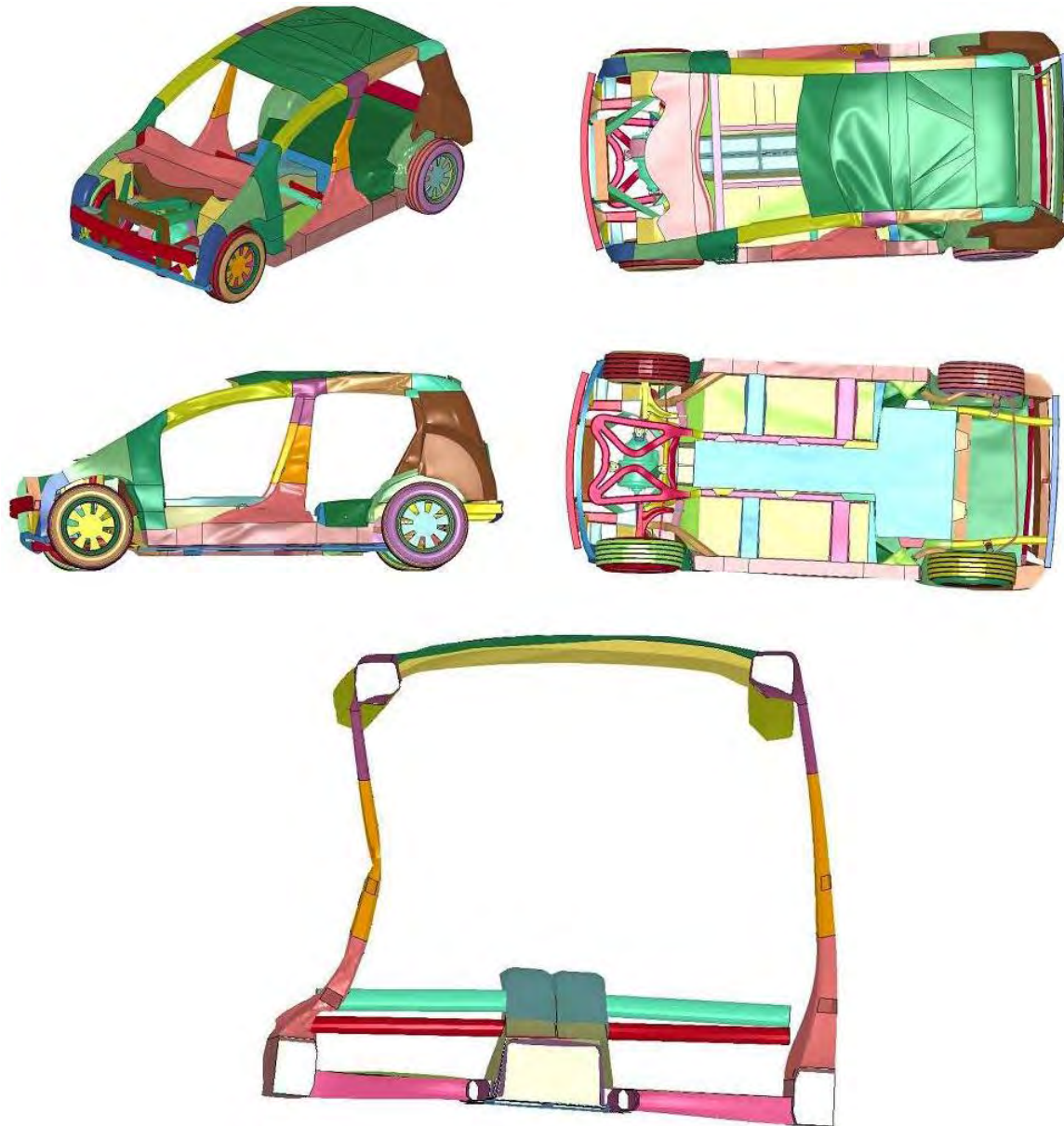
Figure 8.34: IIHS side impact deformed shape : design 60
