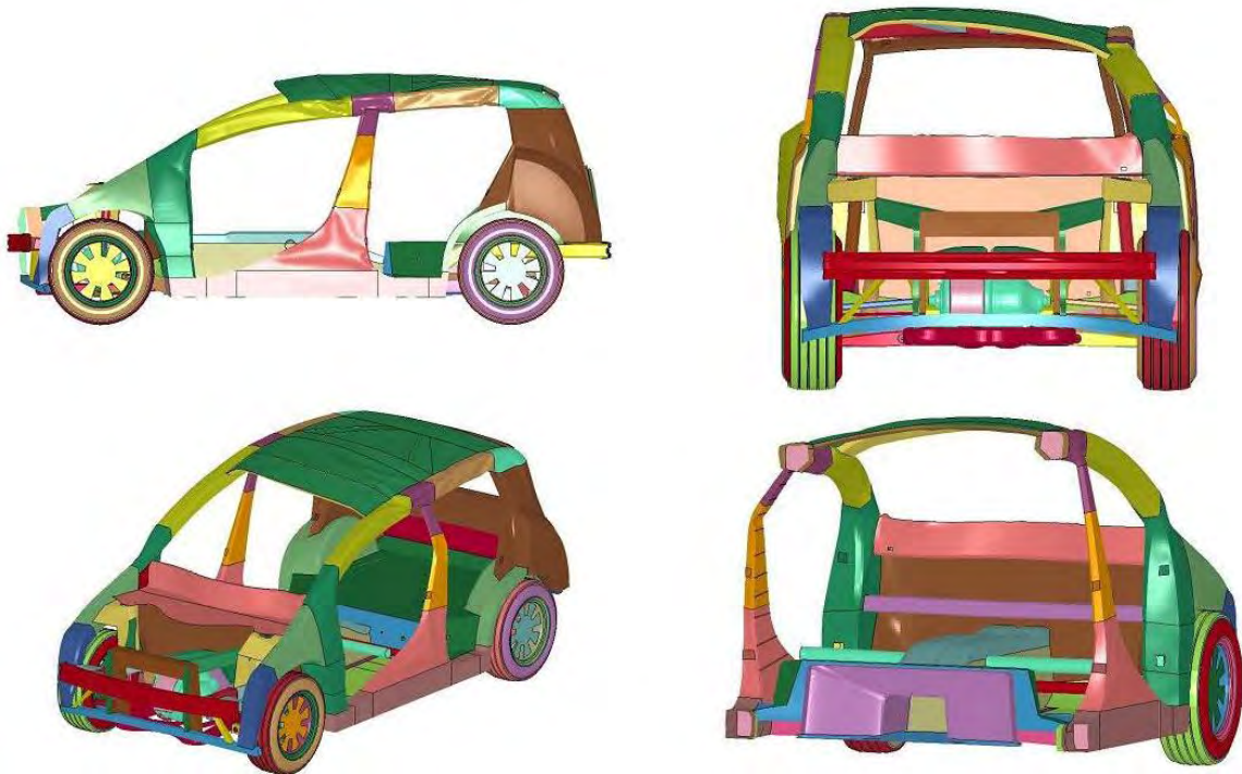
Figure 8.35: Roof crush deformed shape : design 60
