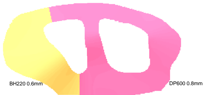
Figure 3.3: Example of a laser weld blank used for a body side panel (FSV body side outer shown)
