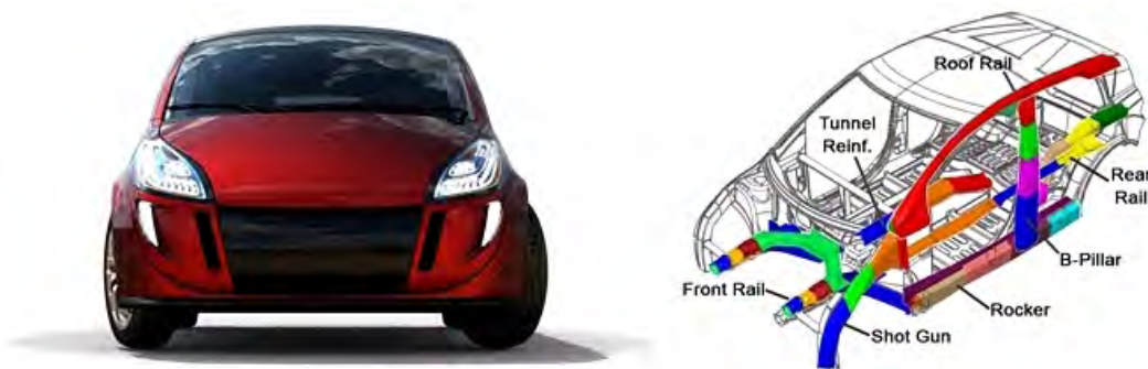
Figure 18.2: FSV BEV; Curb Weight = 958 kg. Body Structure Mass = 187.7 kg
