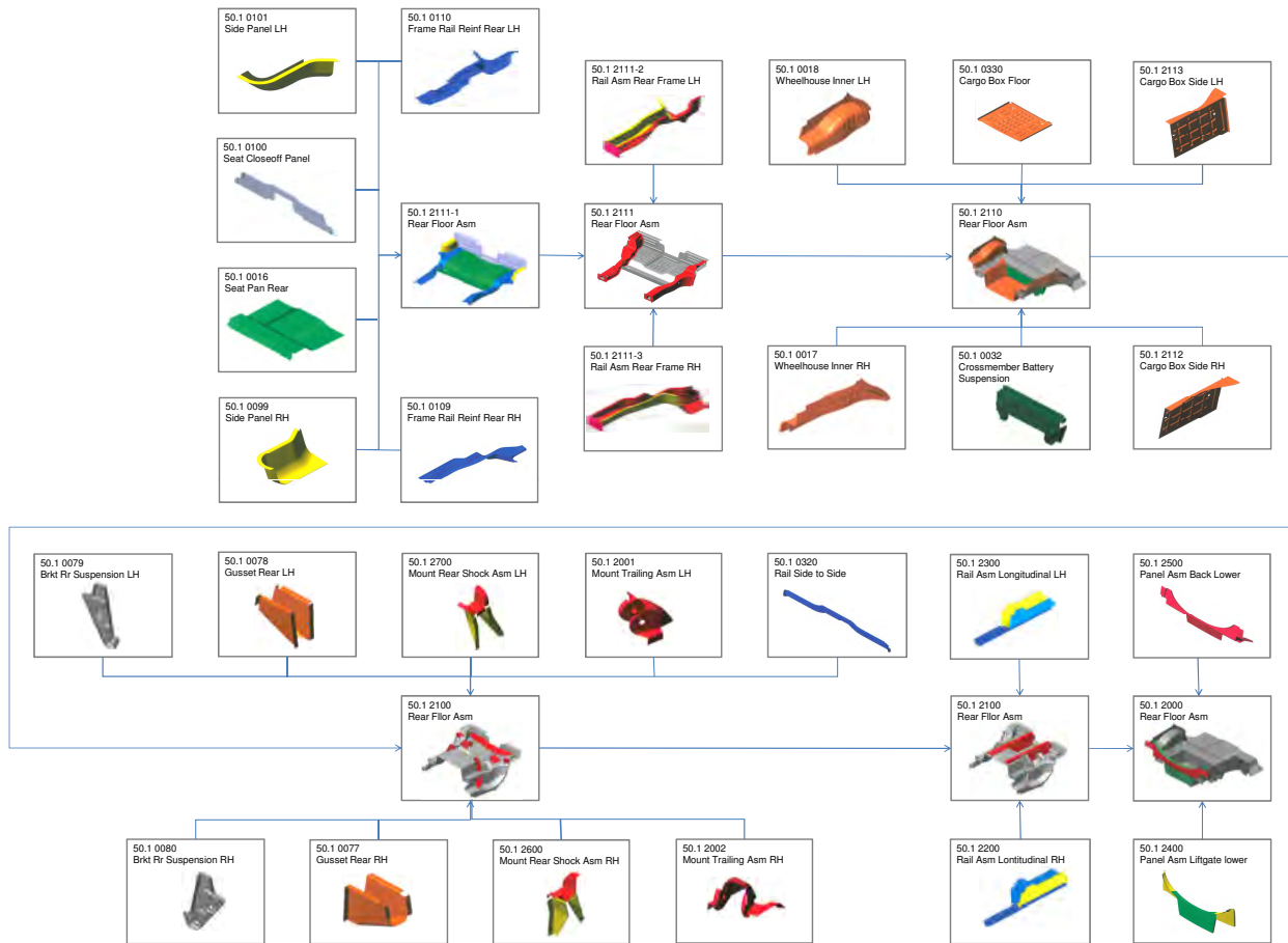
Figure 13.71: Rear floor assembly sequence part diagram
