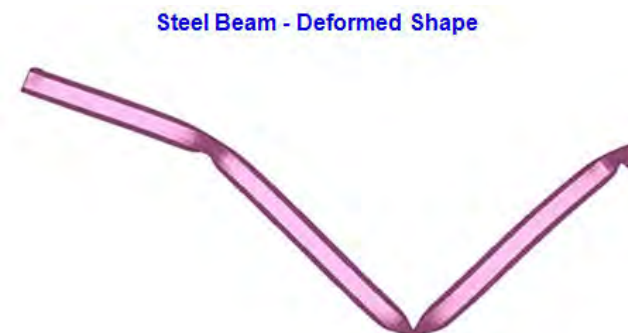
Figure 20.114: Test Beam - Deformed Shape of Steel Version
