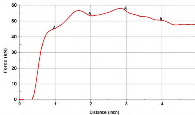
Figure 8.36: Roof crush force-deformation curve : design 60
