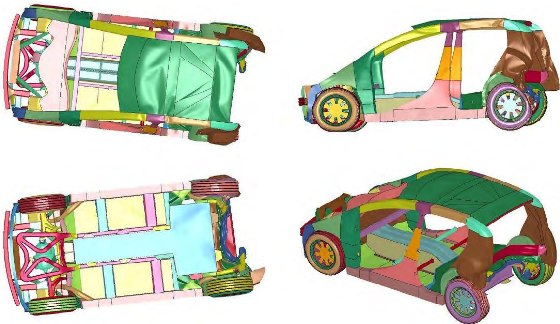
Figure 8.32: Rear offset deformable barrier deformed shape : design 60
