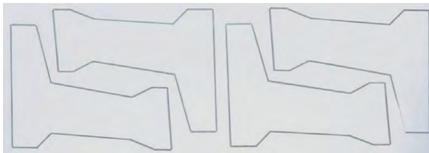
Figure 12.2: FSV B-pillar concept part nesting
