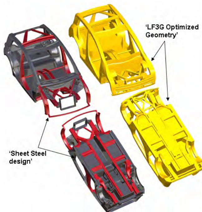
Figure 2.29: FSV body structure comparison - Sheet Steel Design Vs. LF3G Geometry
