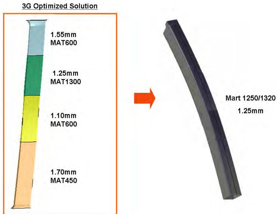
Figure 11.26: B-pillar - closed roll formed solution with stamped B-pillar Outer (not shown)
