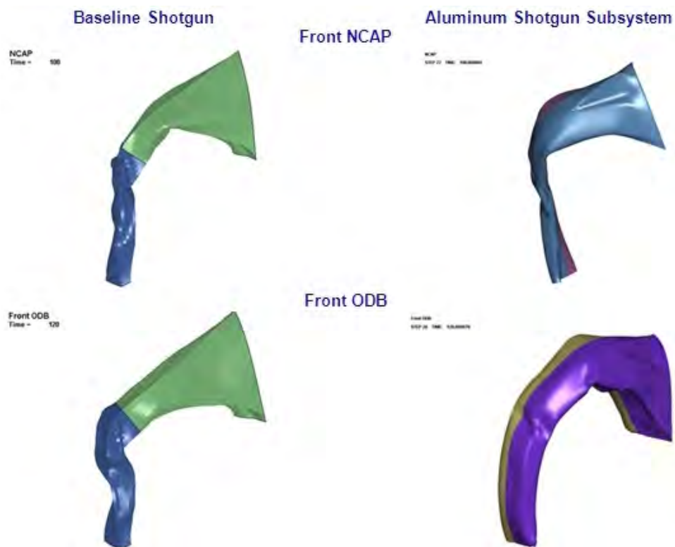
Figure 10.117: Aluminum shotgun design solution - deformation comparison to baseline
