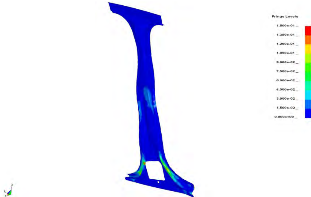
Figure 14.53: US SINCAP - B-pillar inner (% plastic strain contour)
