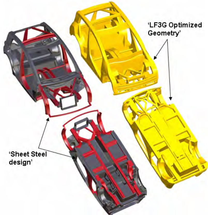
Figure 9.2: FSV body structure comparison - sheet steel design Vs. LF3G geometry
