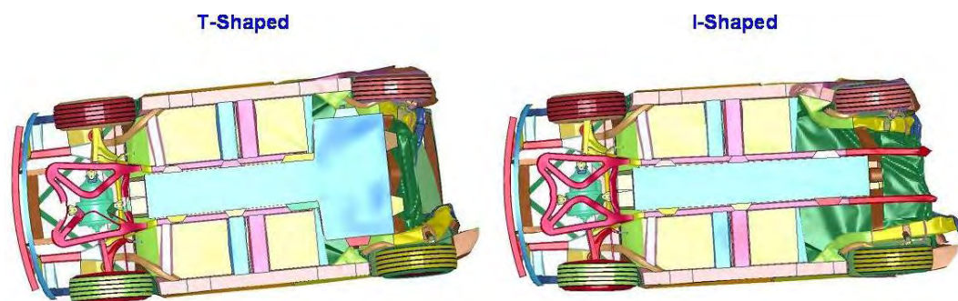
Figure 8.43: T-shape versus I-shape rear impact deformation shape : bottom view
