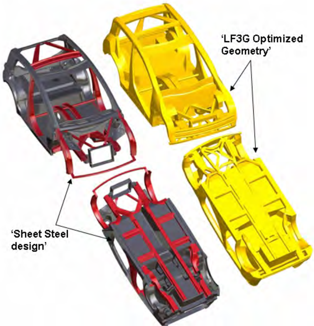
Figure 20.117: FSV body structure comparison - sheet steel design Vs. LF3G geometry
