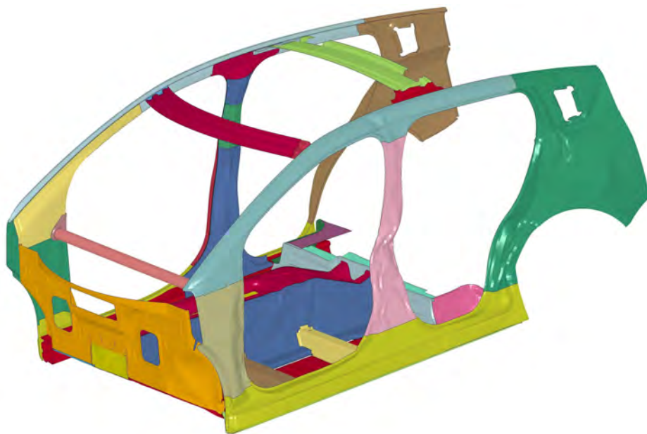
Figure 14.40: IIHS side impact - Structural parts at 100 ms
