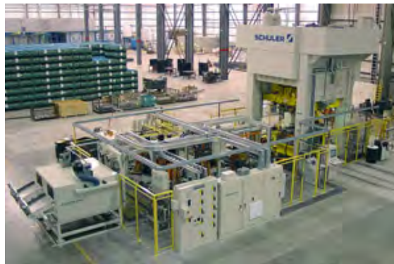
Figure 3.18: Typical example of a hydroforming press (Courtesy: Schuler)
