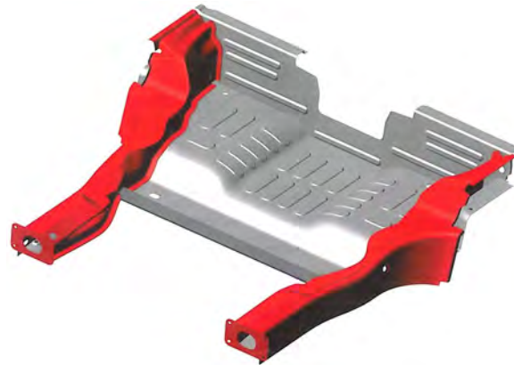
Figure 13.82: 50.1 2111 Rear floor assembly
