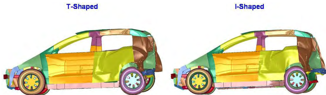
Figure 8.42: T-shape versus I-shape rear impact deformation shape : side view
