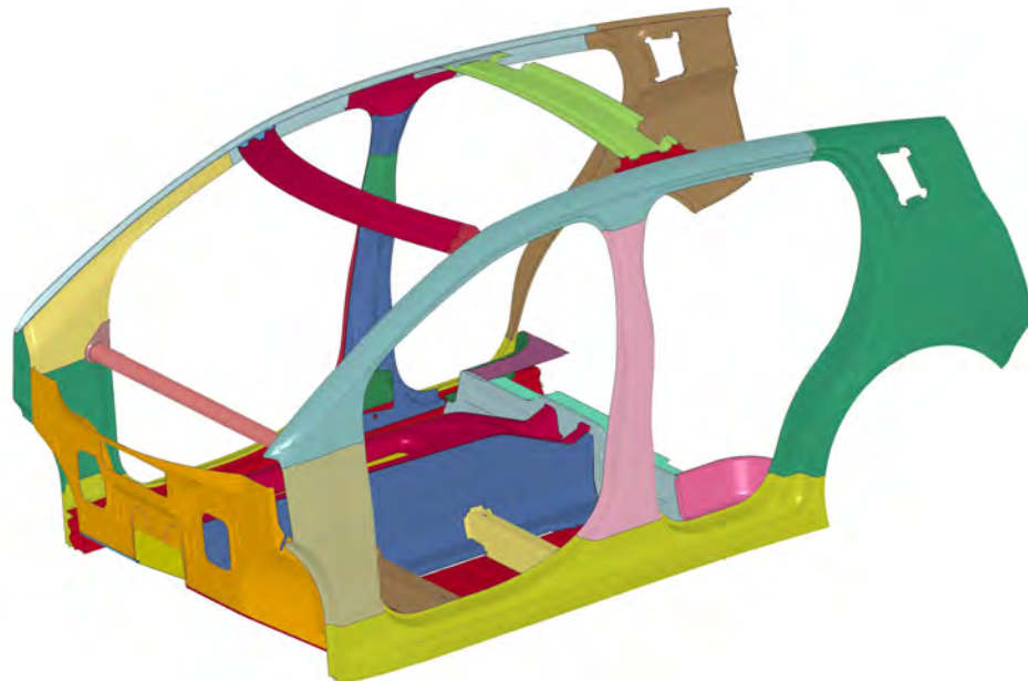
Figure 14.39: IIHS side impact - Structural parts at initial position
