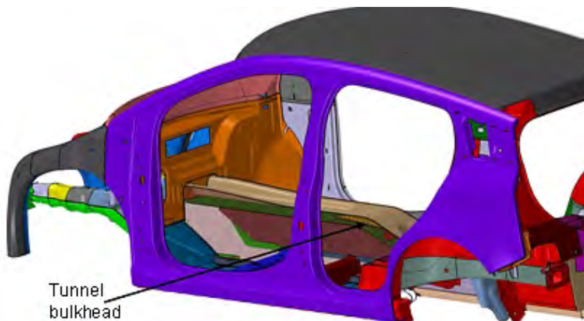
Figure 2.36: Tunnel sub-system shown with the tunnel bulkhead
